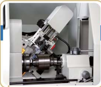
最大研磨螺旋角度 \pm 45^\circ The maximum lead angle in workpiece is \pm 45^\circ
